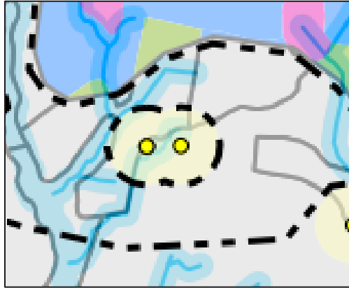
Image 3-1: Example of exclusion within grid connection corridor to avoid residential properties
