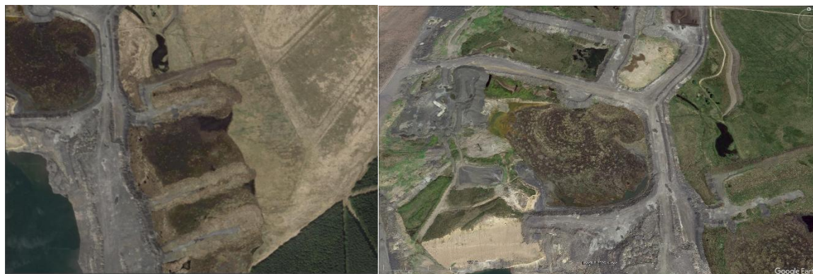
Plate 3-1 Areas of made ground comprising mixed superficial and mining spoil
